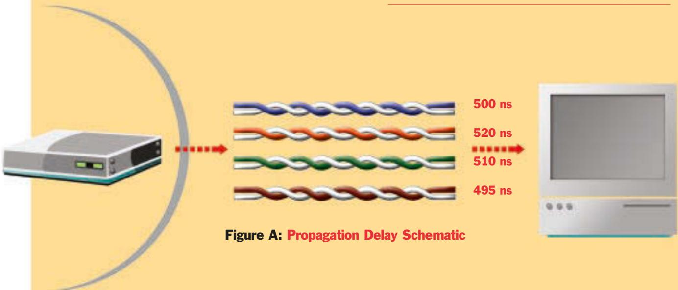
**Figure A: Propagation Delay Schematic**
