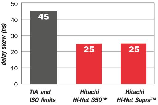
Secondary factors, such as the mechanical and electrical characteristics of the primary copper conductor, also contribute to variances in propagation delay and delay skew performance. Unfortunately, the industry trend has been to design cables with performance headroom built into every transmission parameter except propagation delay and delay skew.
